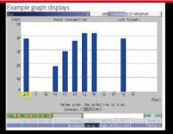
Equipped standard on Citizen lathes, the Eco Monitor shows machine power consumption in the form of a graph. The screens shows various power consumption data points. Working from the I/O screen, this data can be outputted (in CSV format) to a CF card or network.
